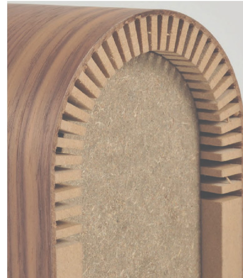
Slots solely in the area of the curvature stabilize the component
