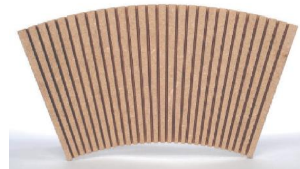
Radial slot cutting in the MDF base material
